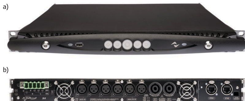
Photo 4: The four-channel X4 offers advanced DSP, WiFi control, and 1,600 W per channel into 8 \Omega (a). The X4 is also bridgeable to two channels at 6,000 W per channel (b).
